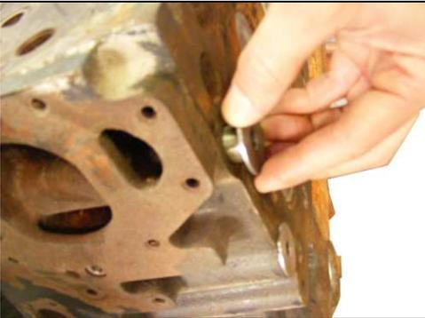
A close-up photograph of a hand turning an Allen bolt to tighten it against the engine head.                                | <p>BASTA SOMENTE UM PEQUENO APERTO NOS 04<br/>PARAFUSOS ALLEN.</p>                                                                  |
