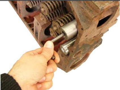
A photograph showing a hand inserting an Allen bolt into the top of the engine head, along with a wedge.                    | <p>O PARAFUSO ALLEN ENTRA JUNTO COM O CALÇO NA<br/>PARTE DE CIMA DO CABEÇOTE.</p>                                                   |
