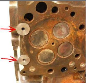
A close-up photograph of the engine head with two red arrows pointing to the installed washers on the head surface.          | <p>NO DETALHE AS PORCAS QUE SÃO INSTALADAS<br/>SOBRE A FACE DO CABEÇOTE, NOS FUIROS DE<br/>FIXAÇÃO DO CABEÇOTE.</p>                 |
